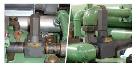
With OEM valves, precise control of air/fuel mixtures can be extremely difficult to adjust. Using a large wrench and cheater bars can be a hassle. CECO truBalance™ Fuel Gas Modulators are easy to install and are designed to accurately control gas flow to each individual power cylinder. Adjustments to the modulator are quickly done by hand.
